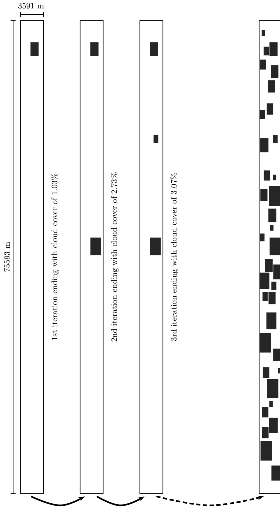
Figure 3.31: The procedure of generating the cloud pattern band using Jewell's method. Black parts are cloud shadows. In this example, the cloud cover is set to be 30% and the cloud velocity is 10 m/s. The simulation time is 2 hours.
