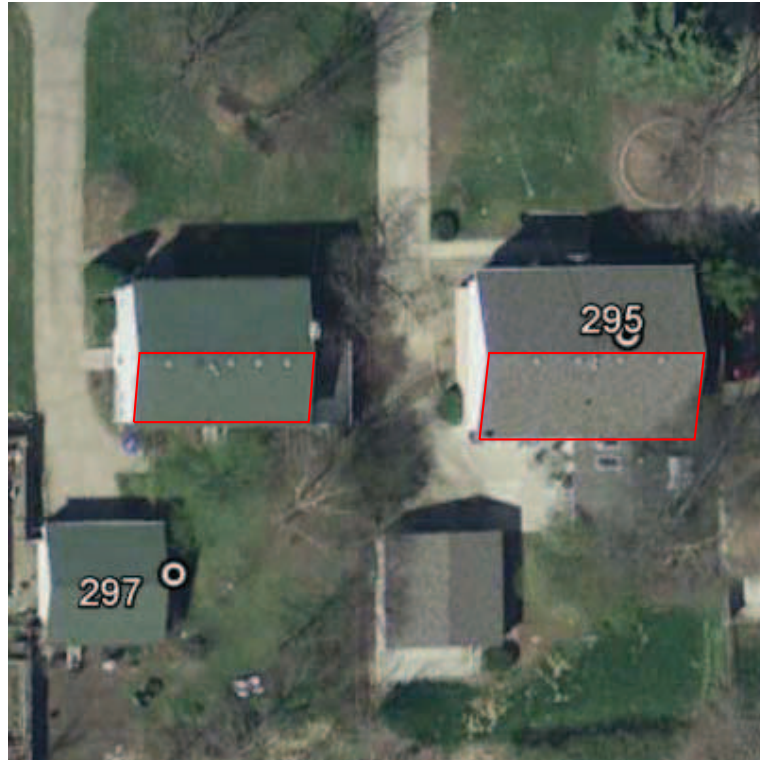
Figure 3.6: Measuring the available roof area for PV system.
